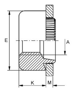
Female thread A = M3Height K = 3.0Outer diameter E = 6.0Plate thickness = 2.6 to 2.8
